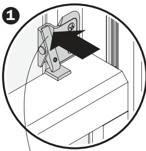
Push top to re-engage window opening control device.
