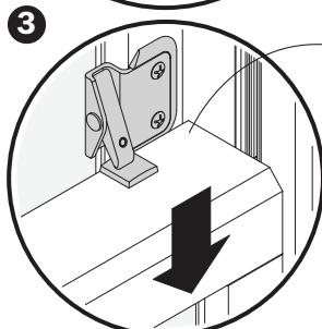
Lower bottom sash. Window opening control devices automatically reset.
