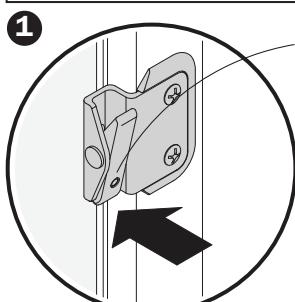
To fully open bottom sash, disengage both window opening control devices by pushing the orange dot.
